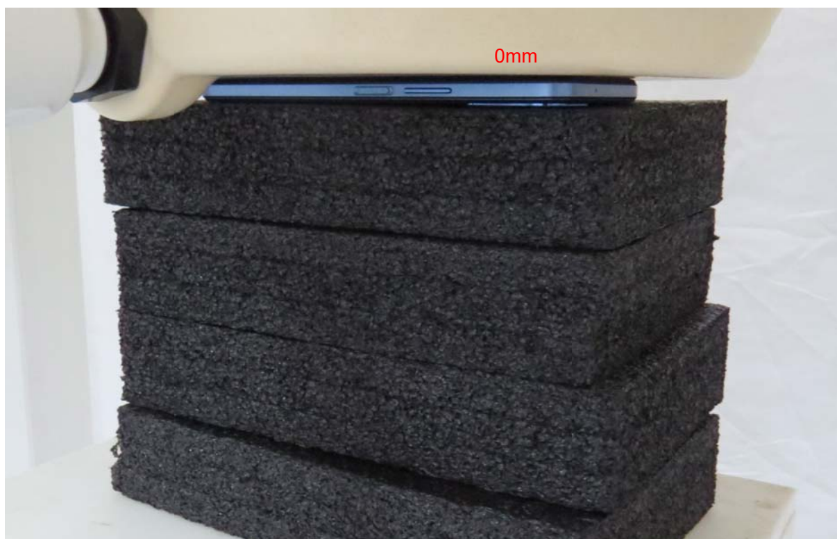
Picture 14: Front Side, the distance from handset to the bottom of the Phantom is 0mm
