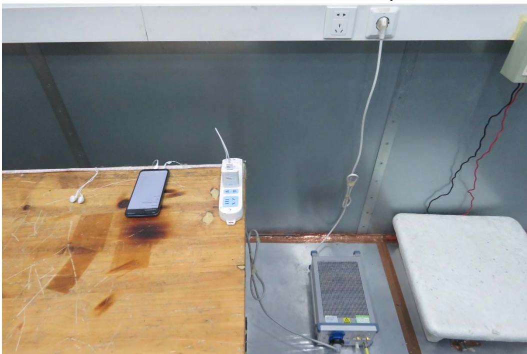
Picture 2 Conducted Emission Test Setup
