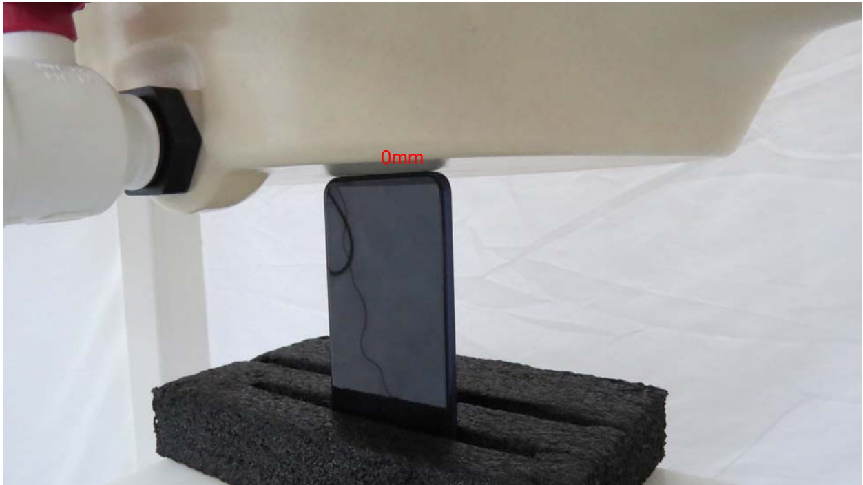
Picture 13: Bottom Edge, the distance from handset to the bottom of the Phantom is 0mm
