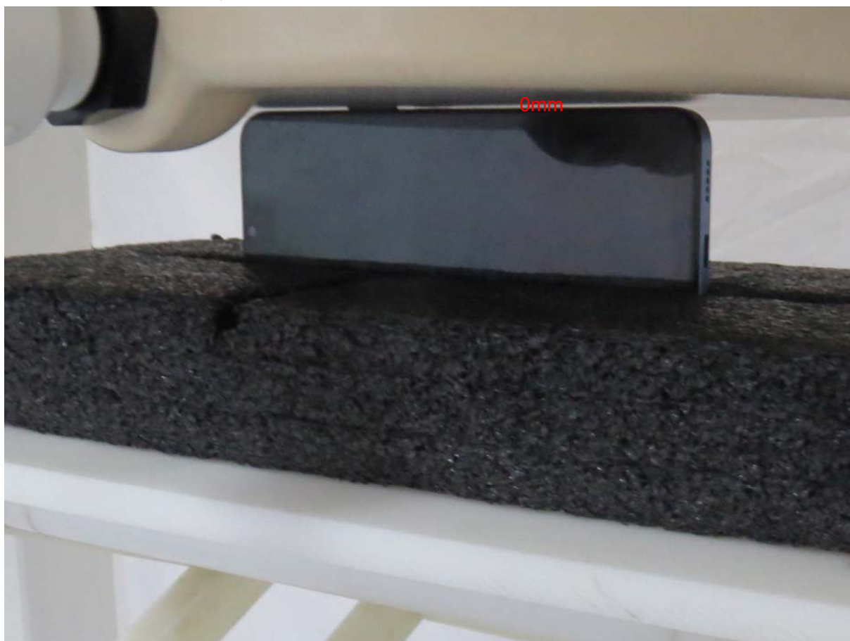
Picture 16: Right Edge, the distance from handset to the bottom of the Phantom is 0mm
