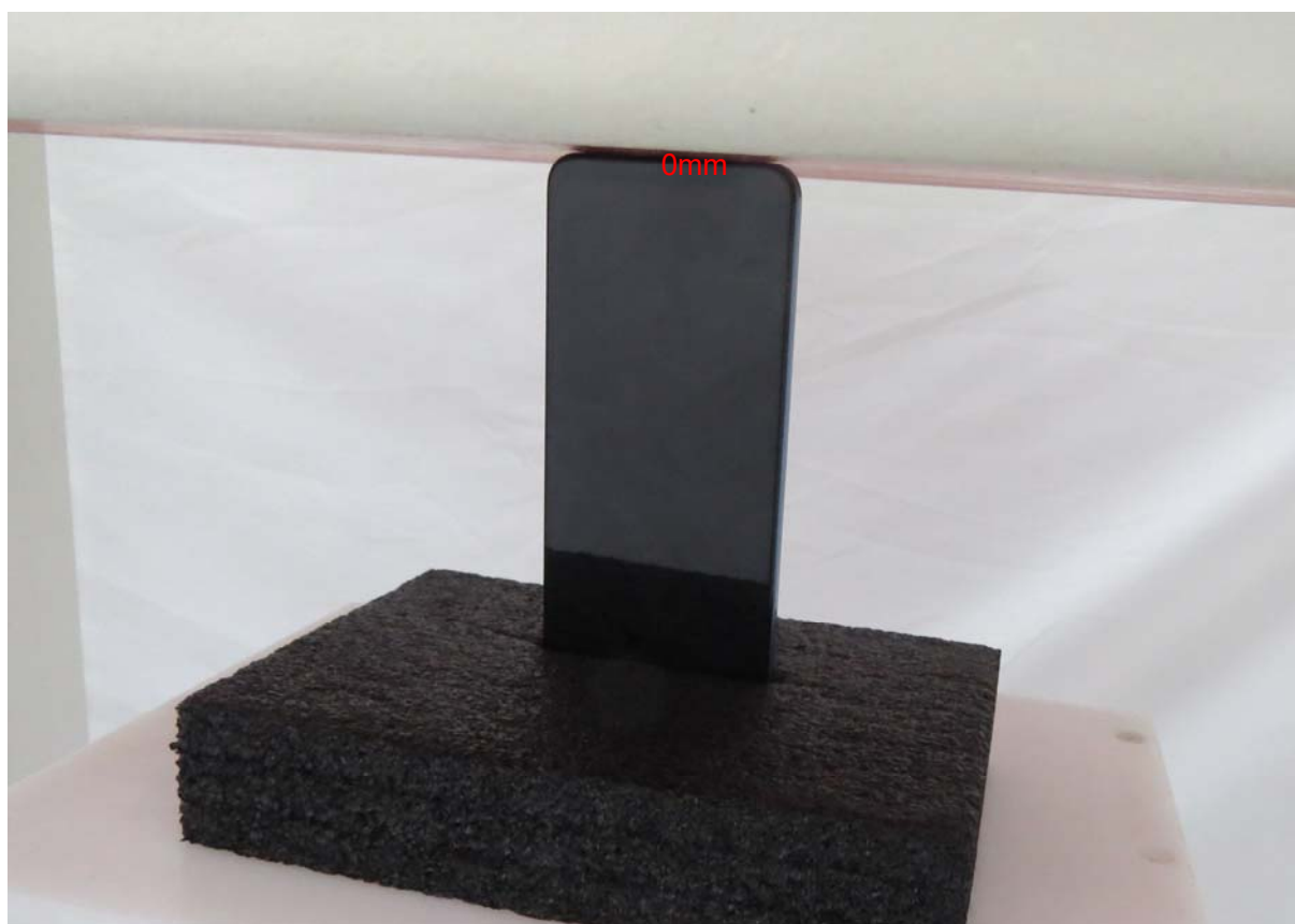
Picture 18: Bottom Edge, the distance from handset to the bottom of the Phantom is 0mm
