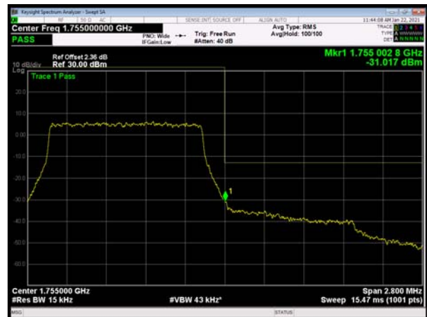
LTE Band 4 QPSK 1.4MHz CH-High, 100%RB
