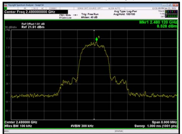
BT 3DH5 CH78, Carrier frequency (MHz): 2480
