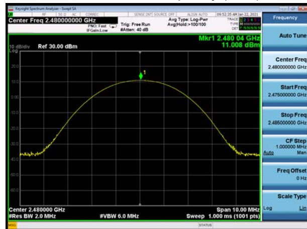
BT DH5 CH78, Carrier frequency (MHz): 2480
