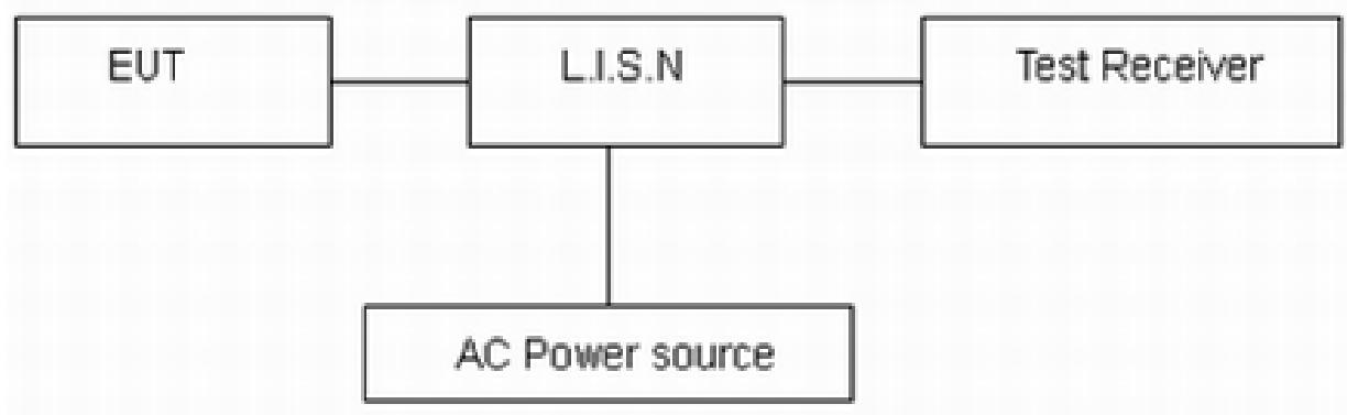
Note: AC Power source is used to 120V/60Hz.
