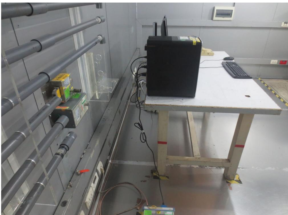
**Radiated Emissions 30 MHz to 1 GHz Test Photos**
