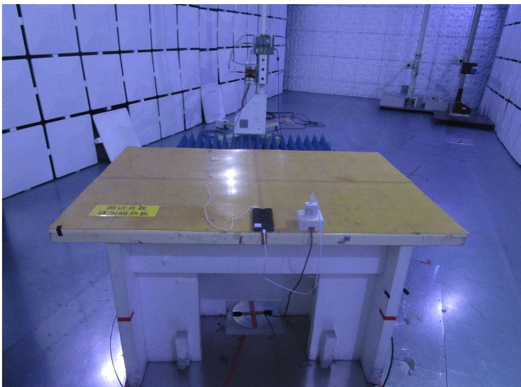
**Mode 11****AC Power Line Conducted Emissions Test Photos**
