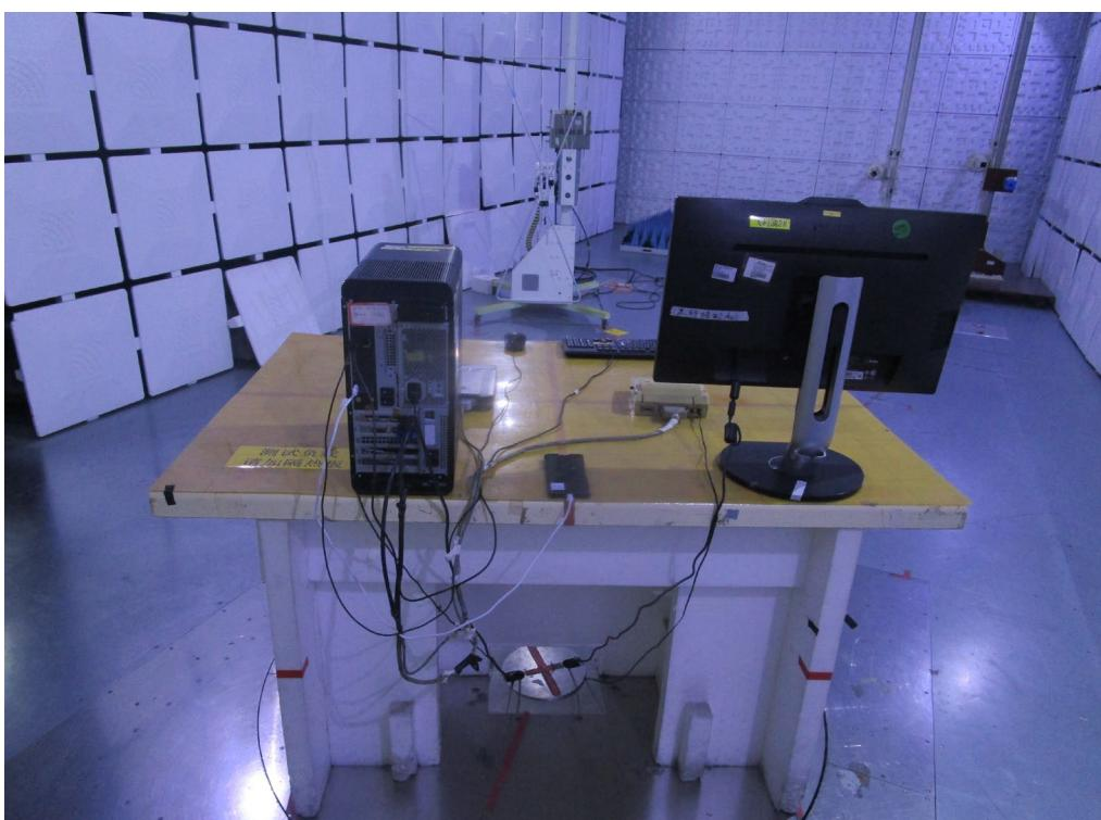
**Radiated Emissions Above 1 GHz Test Photos**
