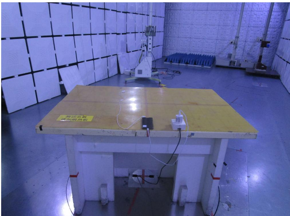
**Radiated Emissions Above 1 GHz Test Photos**
