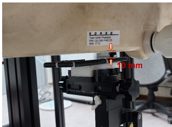
Photograph 15. Hotspot, Back Surface, 10mm
