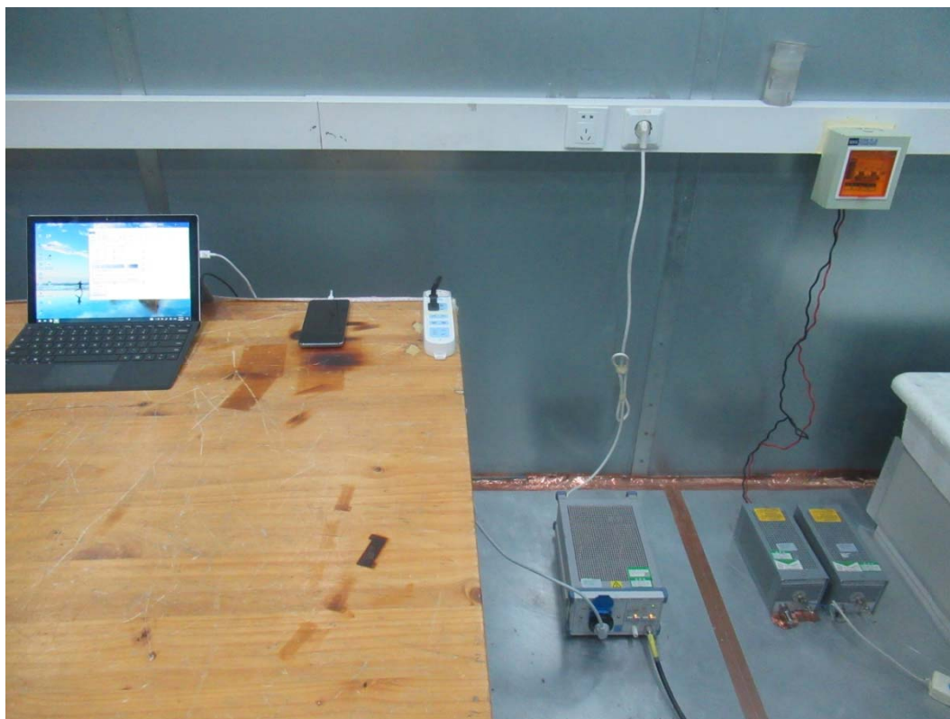
Picture 2: Conducted Emissions Test Setup
