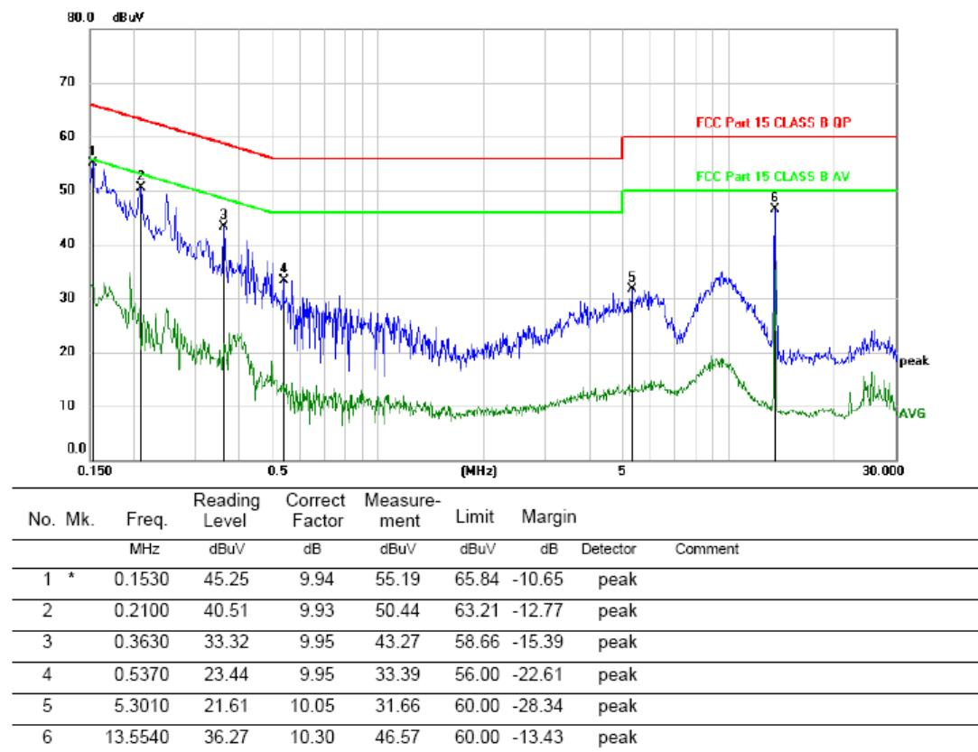
Note: Measurement=Reading Level+Correct Factor. Factor=(LISN or ISN or PLC or Current Probe)Factor+Cable
