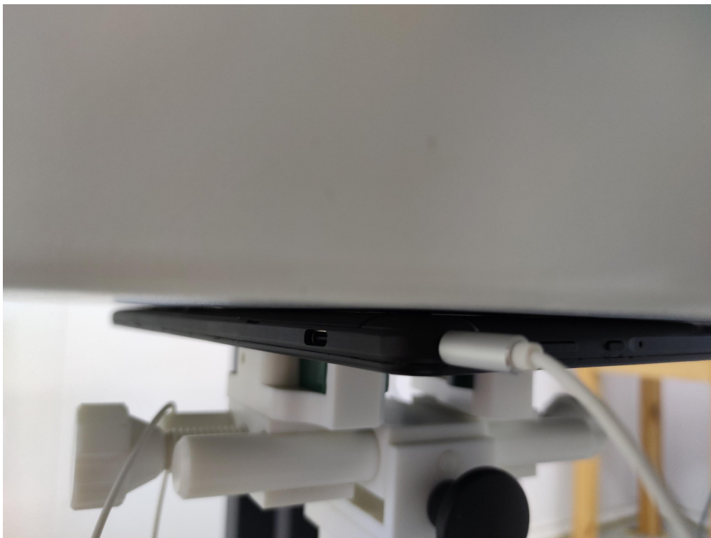
0mm body-worn Back Side Setup Photo (hotspot)
