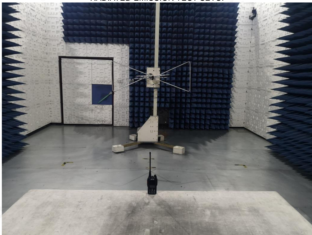
RADIATED EMISSION ABOVE 1G TEST SETUP
