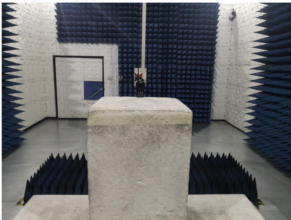
RADIATED EMISSION ABOVE 1G TEST SETUP
