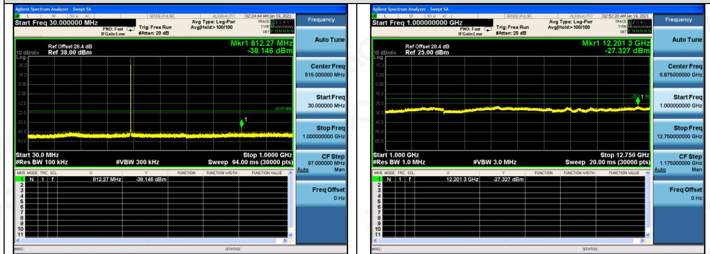
12.5kHz, Analog modulation, Assigned Frequency:435.025MHz, 5W
