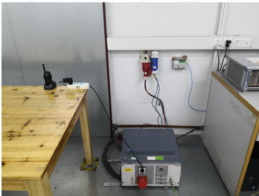
RADIATED EMISSION TEST SETUP-BELOW 1GHZ
