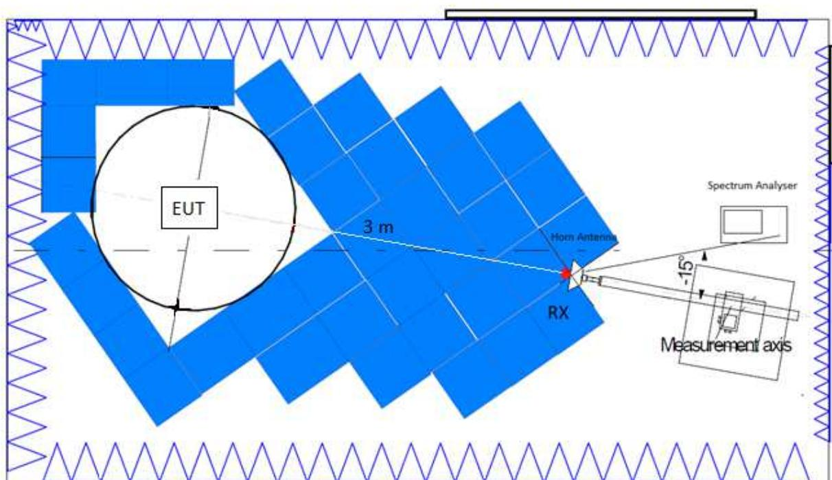
Radiated measurements setup  $f > 17$  GHz up to 26 GHz:
