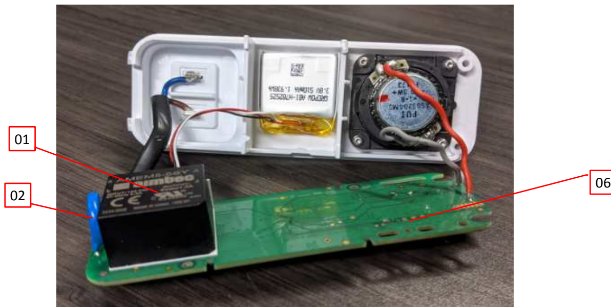
Photo 4 - Internal Bottom view of the SATELLITE PCB and components
