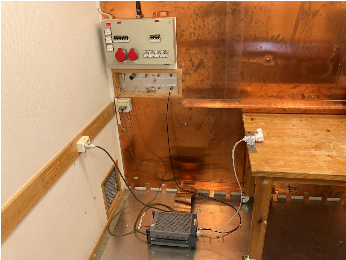
Test setup for conducted emission 150 kHz – 30 MHz
