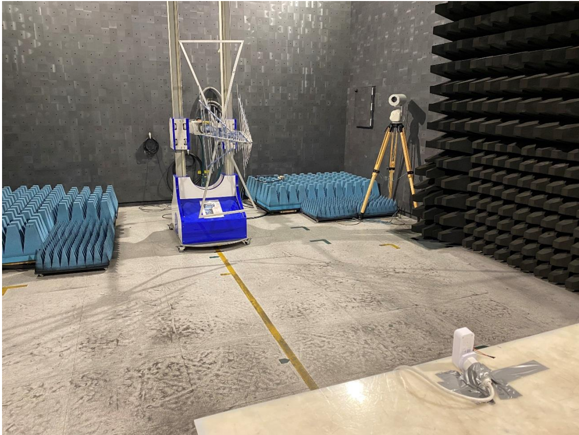
Test set up radiated emission 30 MHz – 1 GHz
