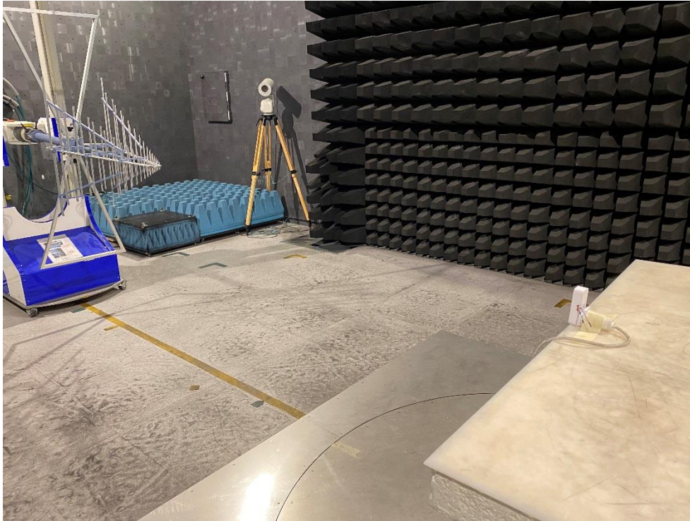
Test set up radiated emission 30 MHz – 1 GHz
