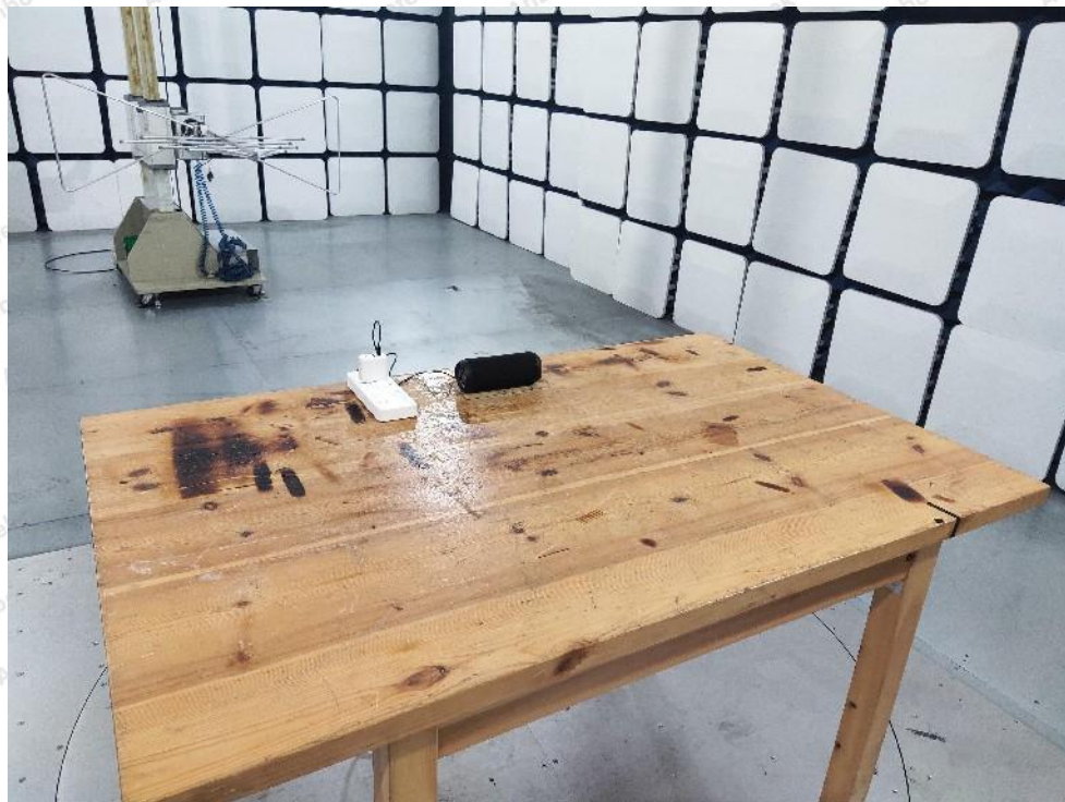
Photo of Radiation Emission Test
