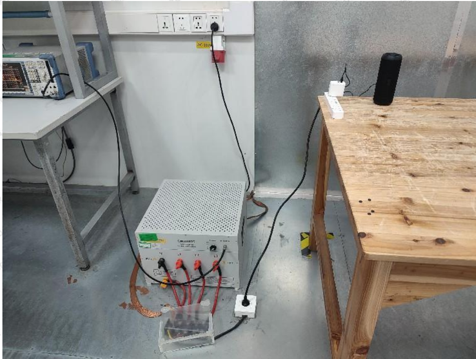
Photo of Conducted Emission Measurement
