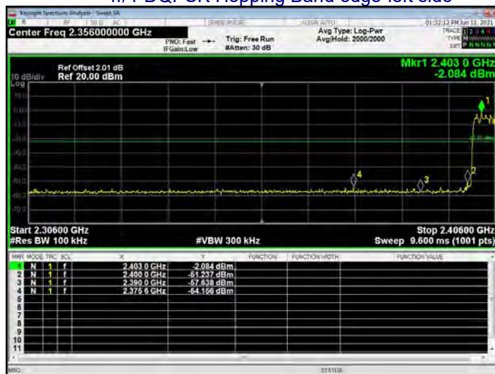
\pi/4 -DQPSK Hopping Band edge-left side
