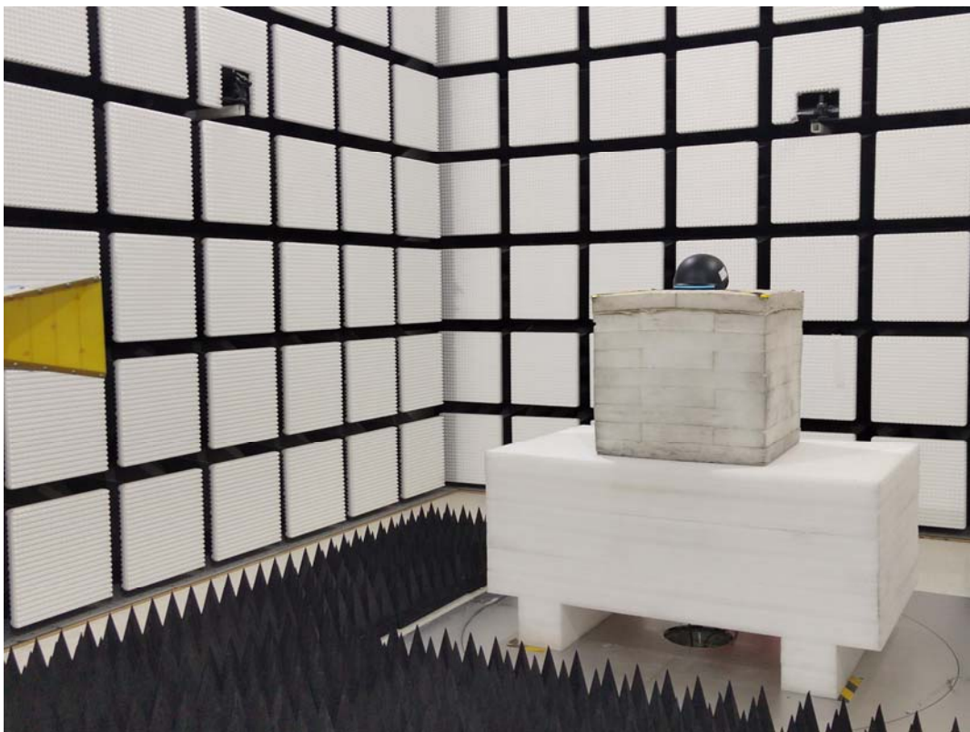
Radiated Emission Above 1GHz View
