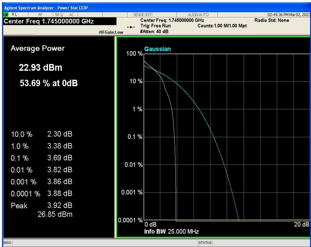
Band66 QPSK BW=10MHz Channel=132622 RB Size=1 Position=#0
