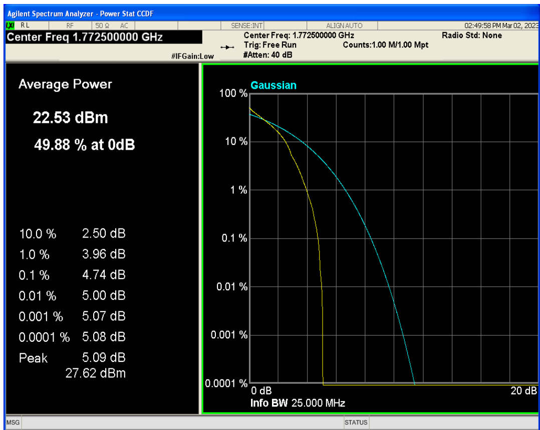
Band66 QPSK BW=20MHz Channel=132072 RB Size=1 Position=#0
