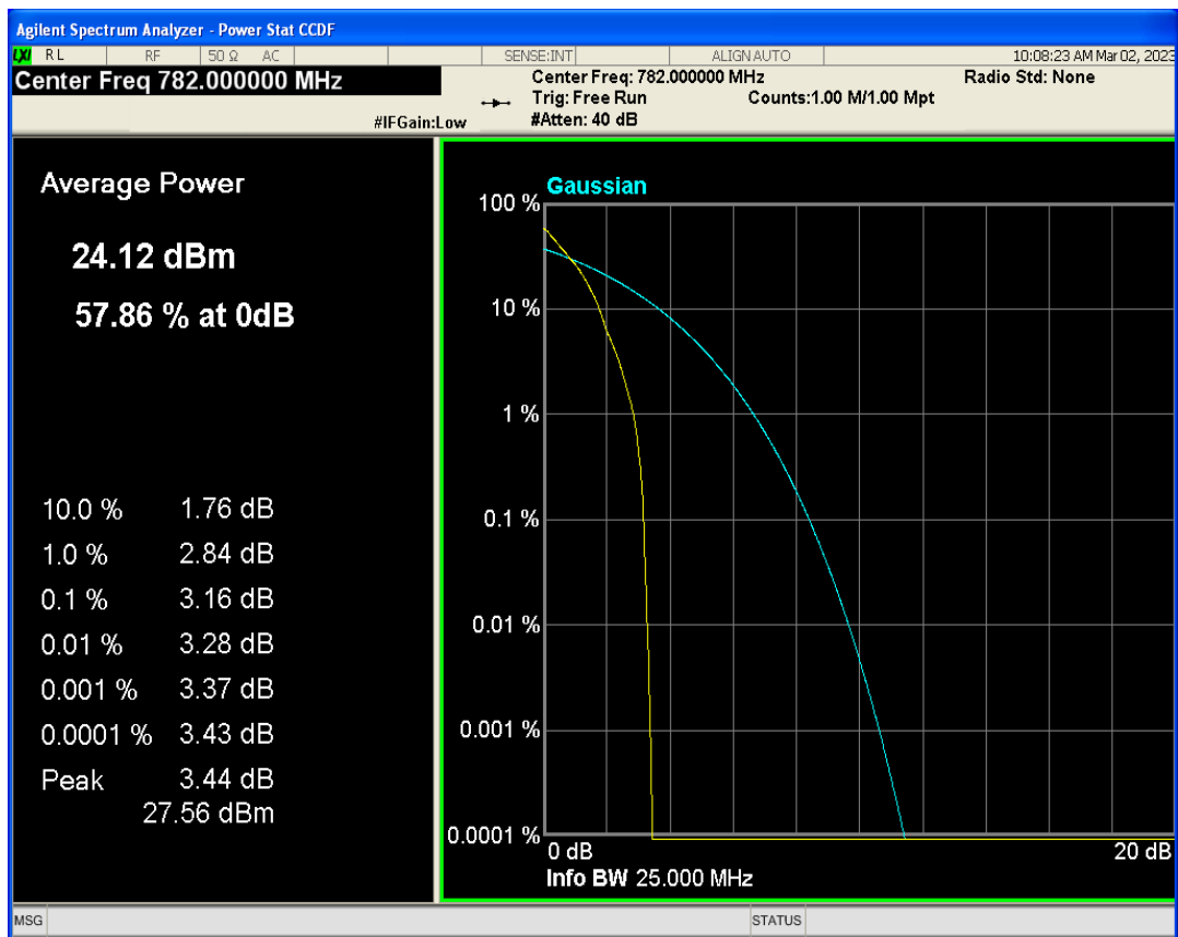
Band13 QPSK BW=5MHz Channel=23205 RB Size=1 Position=#0
