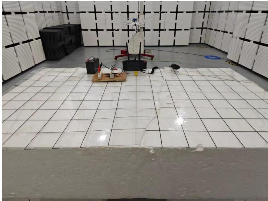
**Set-up for Radiated Emission (RE), Above 1GHz**
