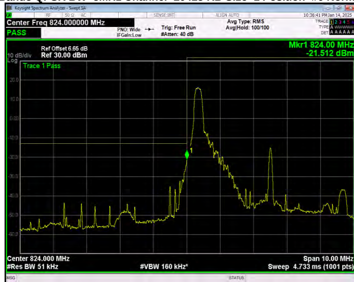
Band5 QPSK BW=5MHz Channel=20425 RB Size=1 Position=#Max Extended
