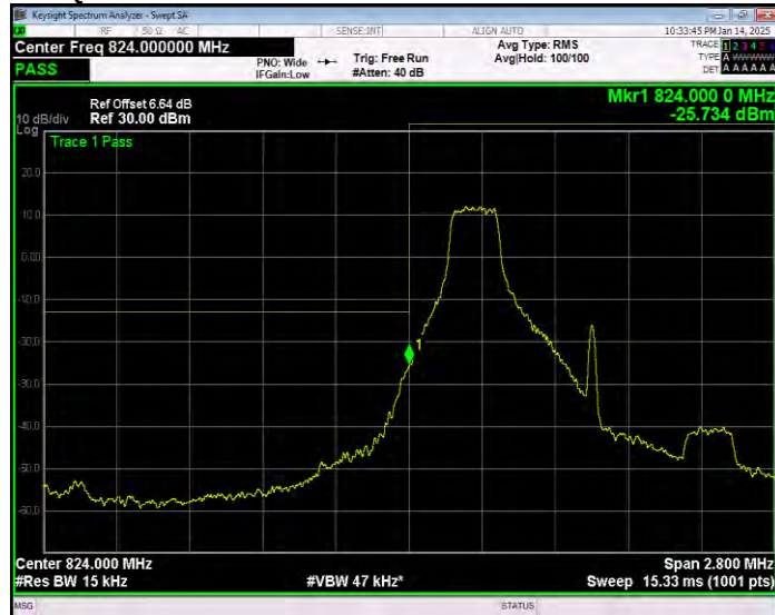
Band5 QPSK BW=1.4MHz Channel=20407 RB Size=1 Position=#Max Extended
