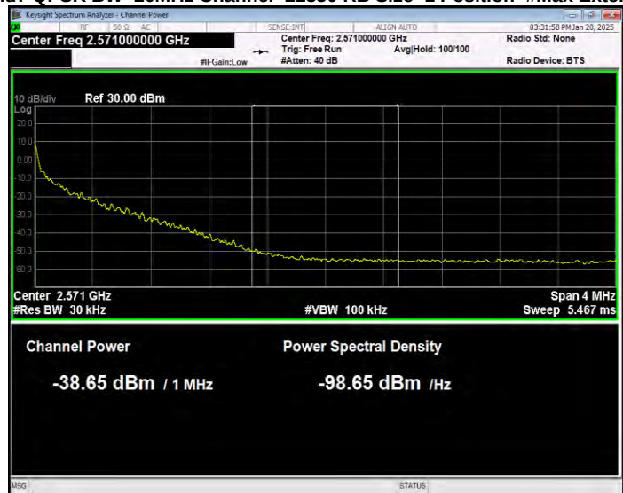
Band7 QPSK BW=20MHz Channel=21350 RB Size=1 Position=#Max Normal
