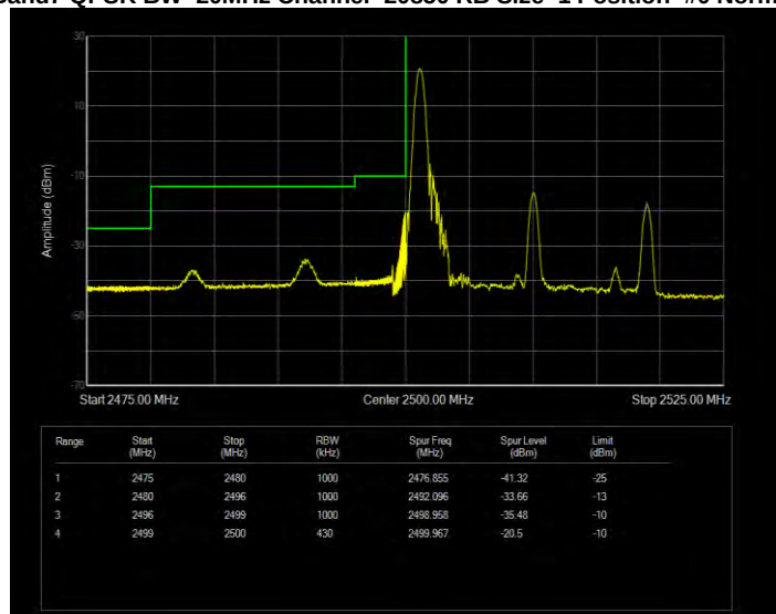
Band7 QPSK BW=20MHz Channel=20850 RB Size=1 Position=#Max Extended
