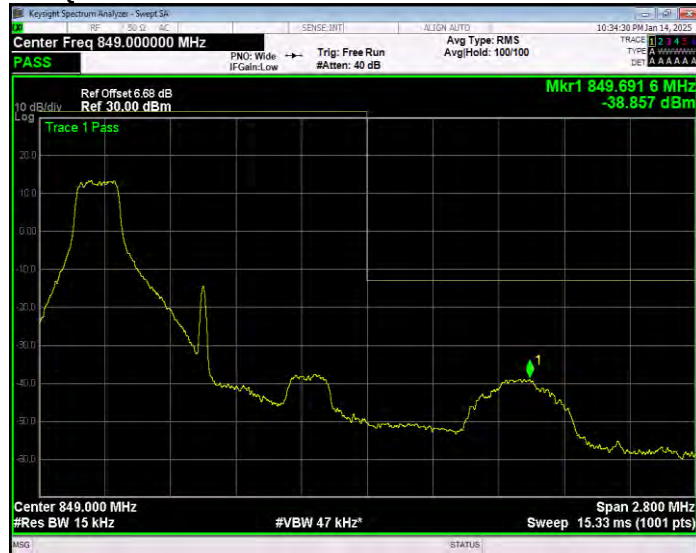
Band5 QPSK BW=1.4MHz Channel=20643 RB Size=1 Position=#Max Extended
