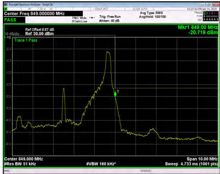
Band5 16QAM BW=5MHz Channel=20625 RB Size=25 Position=#0 Extended
