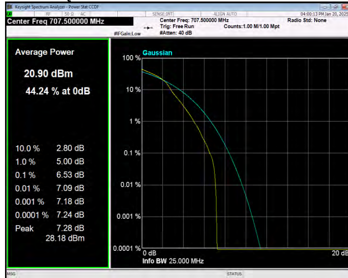
Band12 16QAM BW=10MHz Channel=23130 RB Size=1 Position=#0
