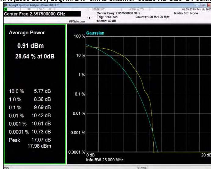
Band40(2350-2360) QPSK BW=10MHz Channel=39200 RB Size=1 Position=#0
