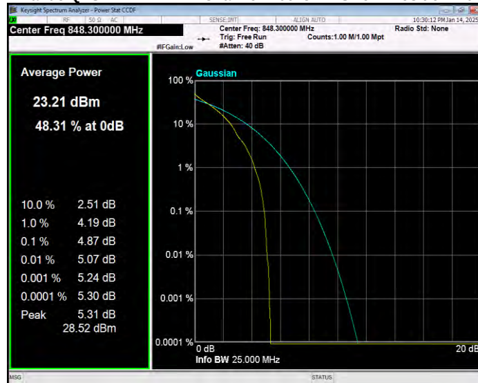
Band5 QPSK BW=10MHz Channel=20450 RB Size=1 Position=#0
