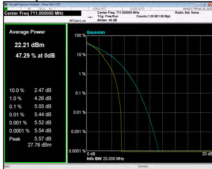
Band12 QPSK BW=3MHz Channel=23025 RB Size=1 Position=#0
