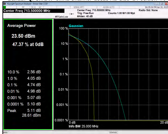
Band38 16QAM BW=10MHz Channel=37800 RB Size=1 Position=#0
