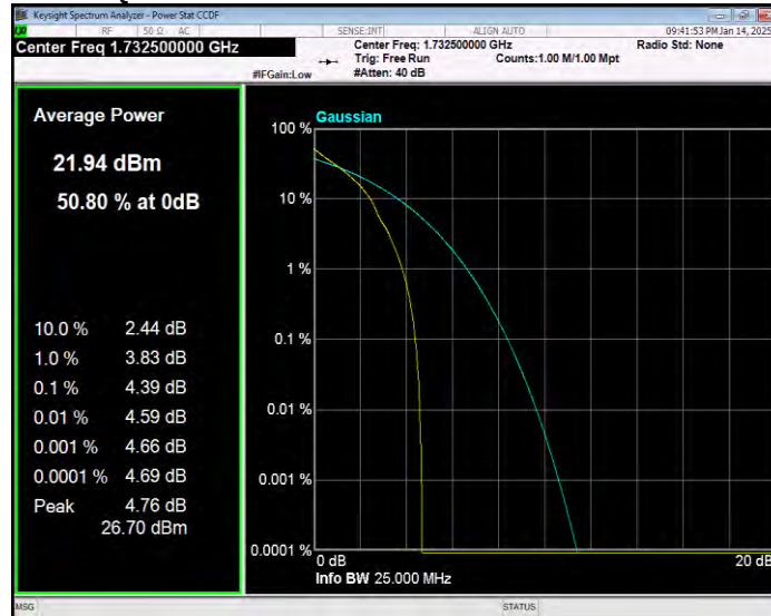
Band4 QPSK BW=1.4MHz Channel=20393 RB Size=1 Position=#0
