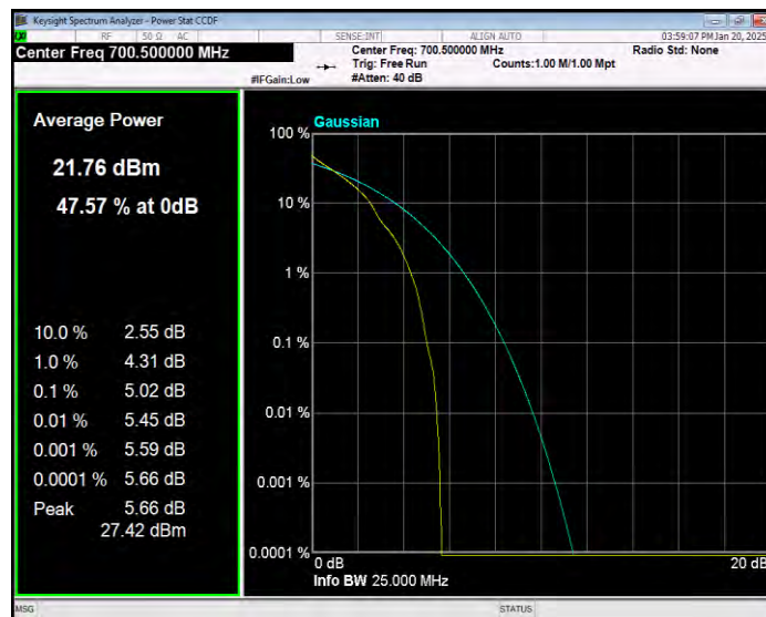
Band12 QPSK BW=3MHz Channel=23095 RB Size=1 Position=#0
