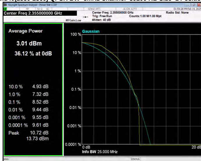
Band40(2350-2360) QPSK BW=5MHz Channel=39225 RB Size=1 Position=#0
