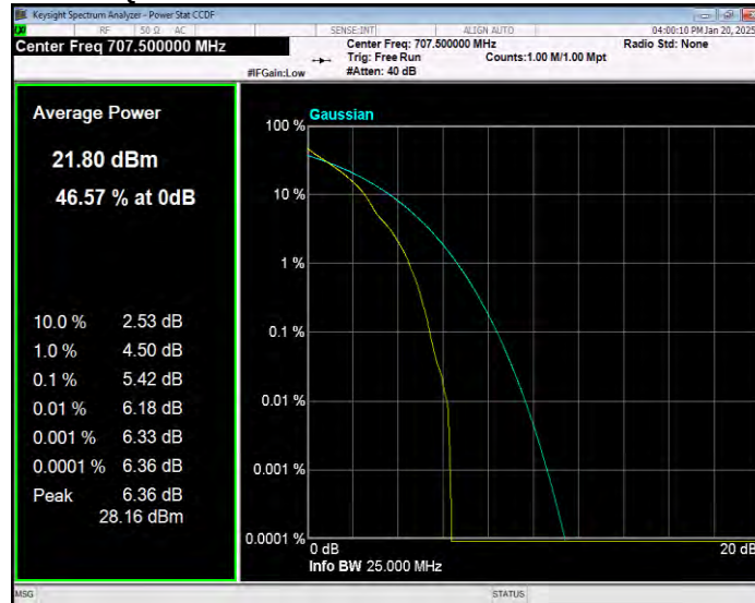
Band12 QPSK BW=10MHz Channel=23130 RB Size=1 Position=#0
