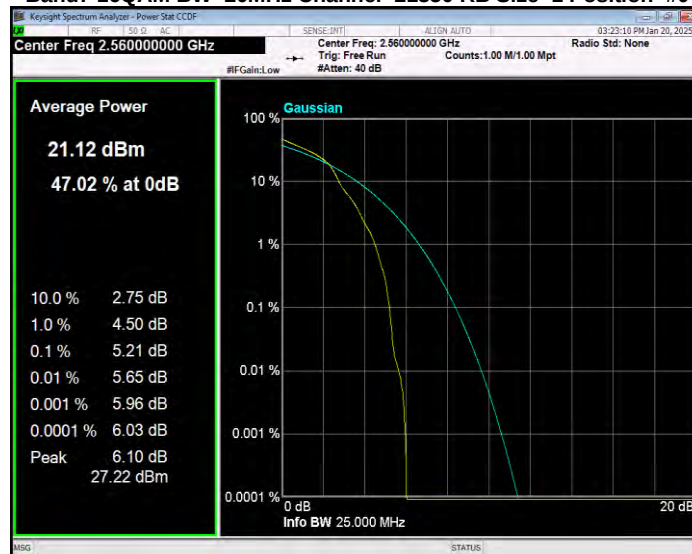
Band7 16QAM BW=5MHz Channel=20775 RB Size=1 Position=#0
