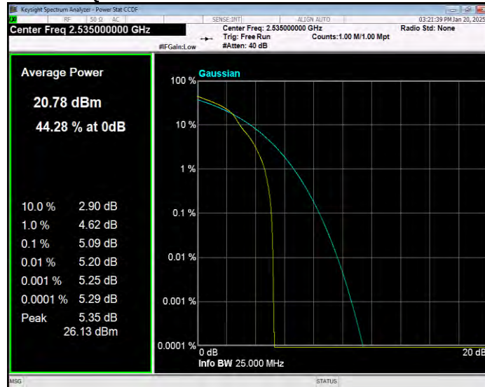
Band7 16QAM BW=5MHz Channel=21425 RB Size=1 Position=#0
