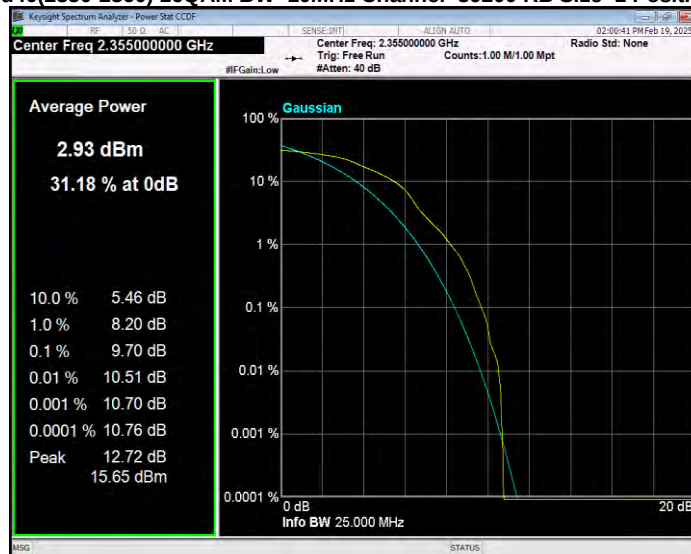
Band40(2350-2360) 16QAM BW=5MHz Channel=39175 RB Size=1 Position=#0
