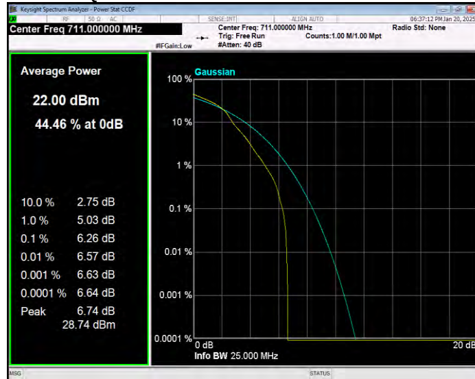
Band17 16QAM BW=5MHz Channel=23755 RB Size=1 Position=#0
