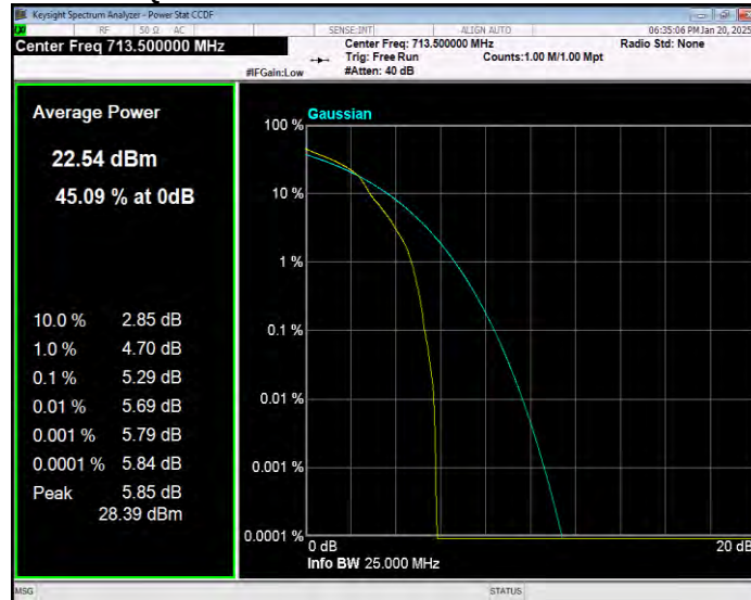
Band17 QPSK BW=10MHz Channel=23780 RB Size=1 Position=#0
