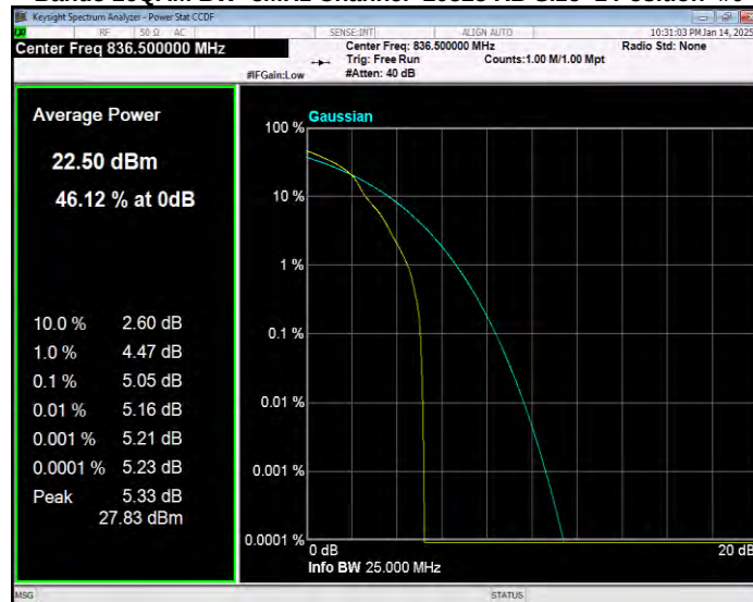
Band5 16QAM BW=5MHz Channel=20625 RB Size=1 Position=#0
