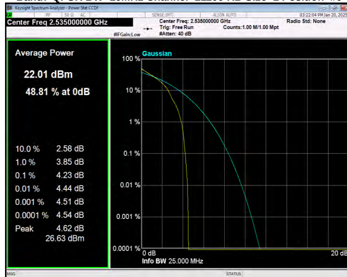
Band7 QPSK BW=10MHz Channel=21400 RB Size=1 Position=#0
