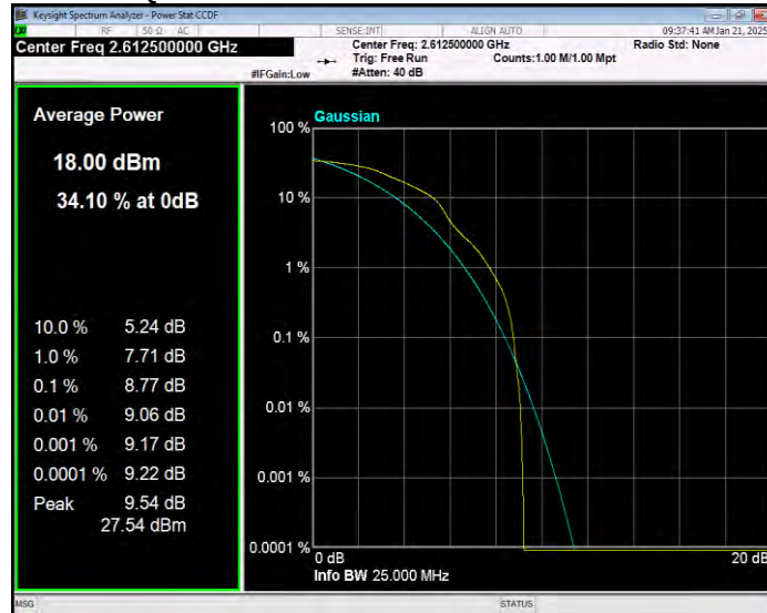
Band38 16QAM BW=20MHz Channel=37850 RB Size=1 Position=#0
