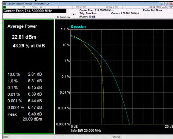
Band12 16QAM BW=5MHz Channel=23035 RB Size=1 Position=#0
