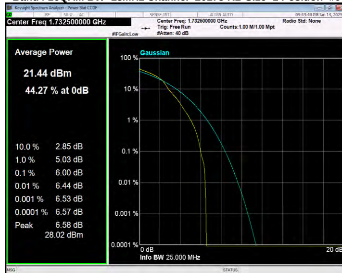
Band4 16QAM BW=15MHz Channel=20325 RB Size=1 Position=#0
