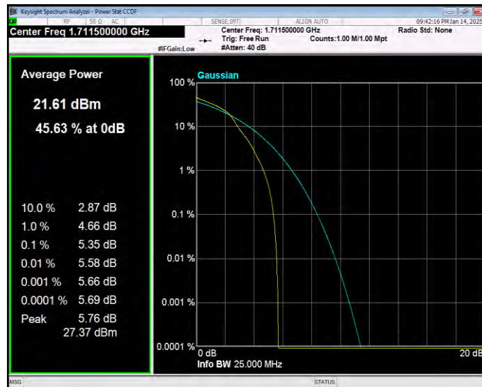
Band4 16QAM BW=3MHz Channel=20175 RB Size=1 Position=#0
