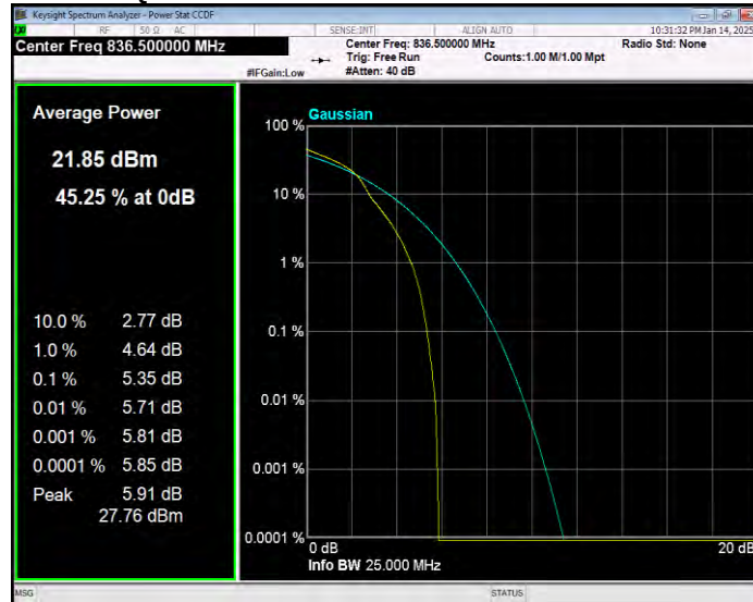
Band5 16QAM BW=10MHz Channel=20600 RB Size=1 Position=#0
