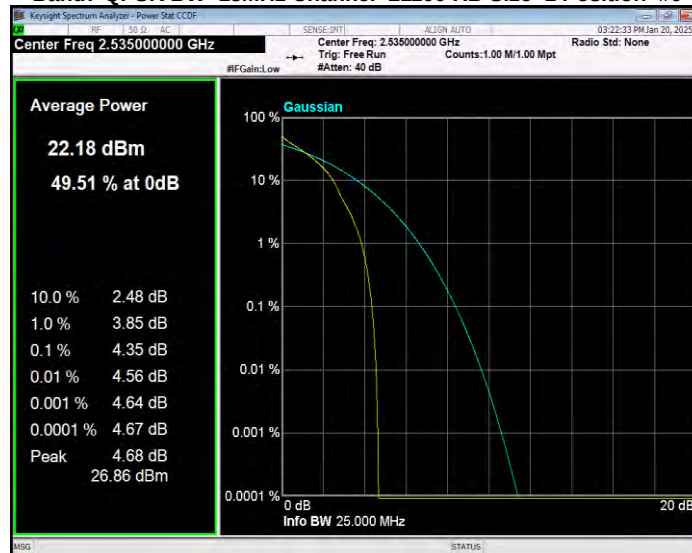
Band7 QPSK BW=15MHz Channel=21375 RB Size=1 Position=#0
