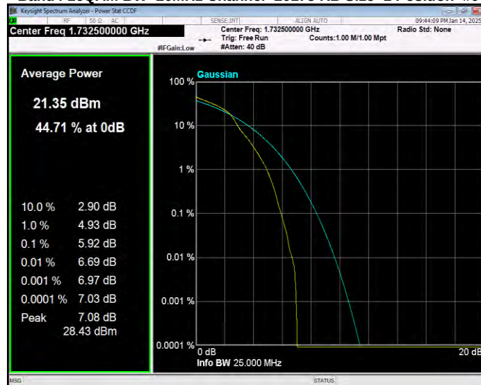
Band4 16QAM BW=20MHz Channel=20300 RB Size=1 Position=#0
