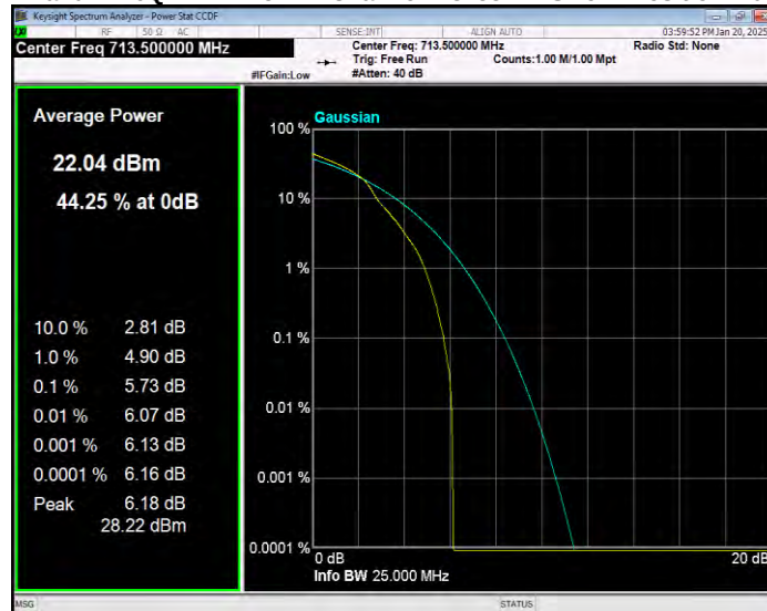
Band12 QPSK BW=1.4MHz Channel=23017 RB Size=1 Position=#0
