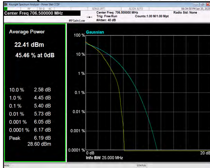
Band17 QPSK BW=5MHz Channel=23790 RB Size=1 Position=#0
