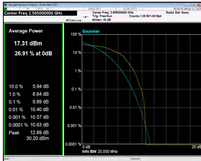
Band38 16QAM BW=5MHz Channel=38225 RB Size=1 Position=#0
