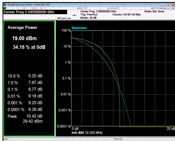
Band38 16QAM BW=10MHz Channel=38200 RB Size=1 Position=#0
