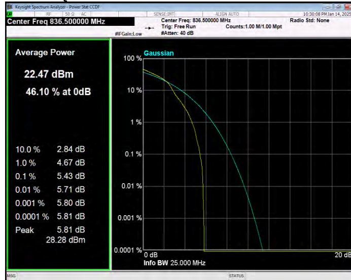
Band5 16QAM BW=1.4MHz Channel=20643 RB Size=1 Position=#0
