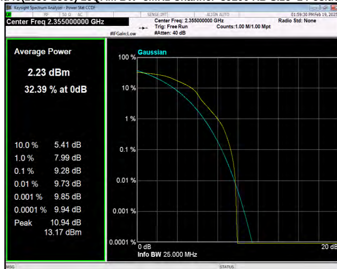
Band40(2350-2360) 16QAM BW=5MHz Channel=39225 RB Size=1 Position=#0
