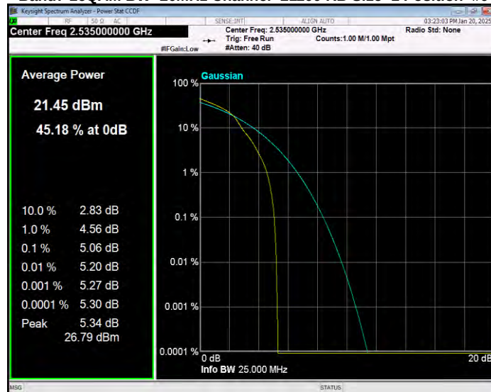
Band7 16QAM BW=20MHz Channel=21350 RB Size=1 Position=#0
