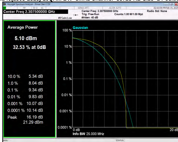
Band40(2305-2315) 16QAM BW=5MHz Channel=38750 RB Size=1 Position=#0
