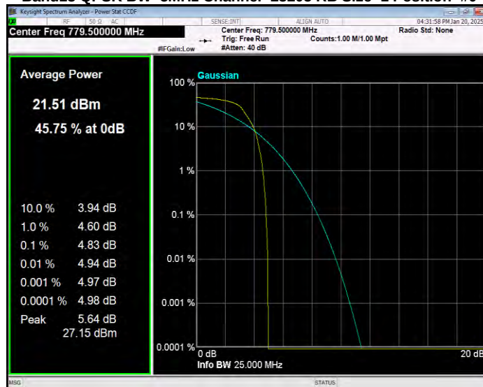
Band13 QPSK BW=5MHz Channel=23230 RB Size=1 Position=#0
