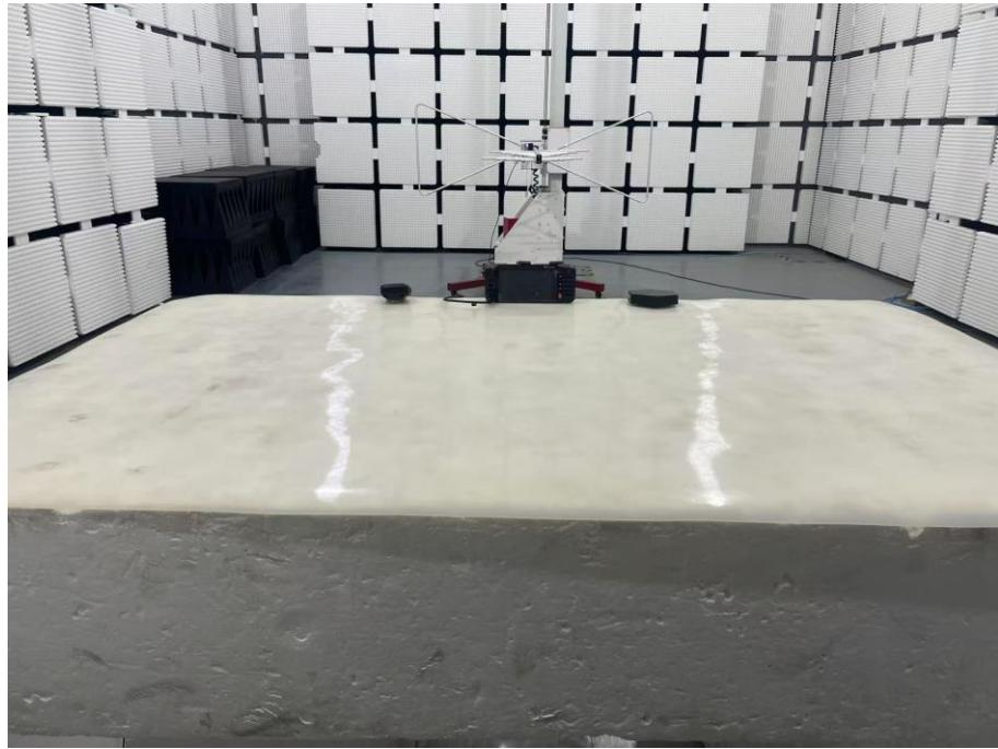
**Set-up for Radiated Emission (RE), Above 1GHz**
