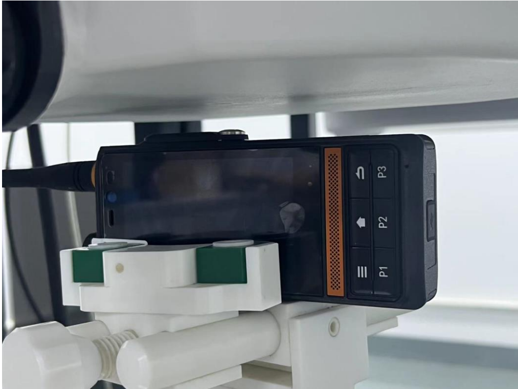
Body Right side (separation distance is 10mm)
