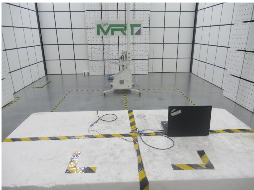
Description: Radiated Spurious Emission Test Setup for Above 1GHz(High Rate)
