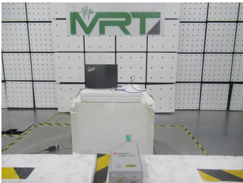
Description: Radiated Spurious Emission Test Setup for Between
