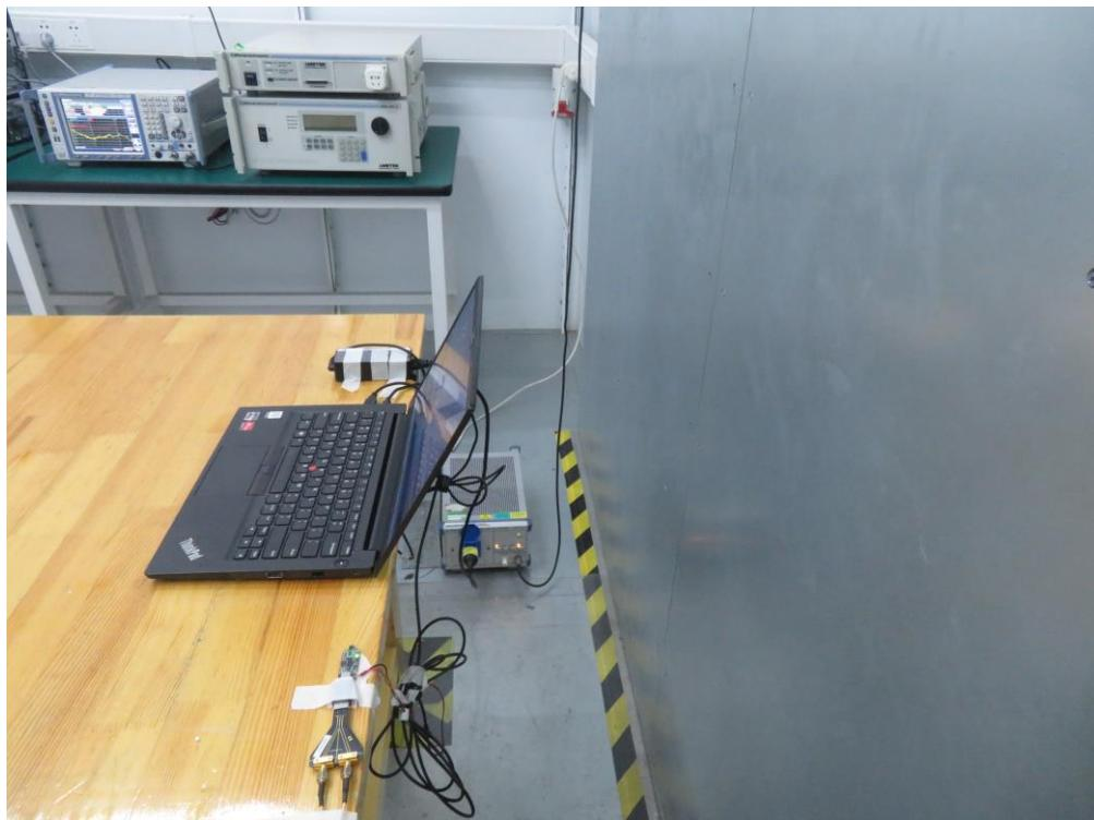
Description: Radiated Spurious Emission Test Setup for Below 30MHz(High Rate)
