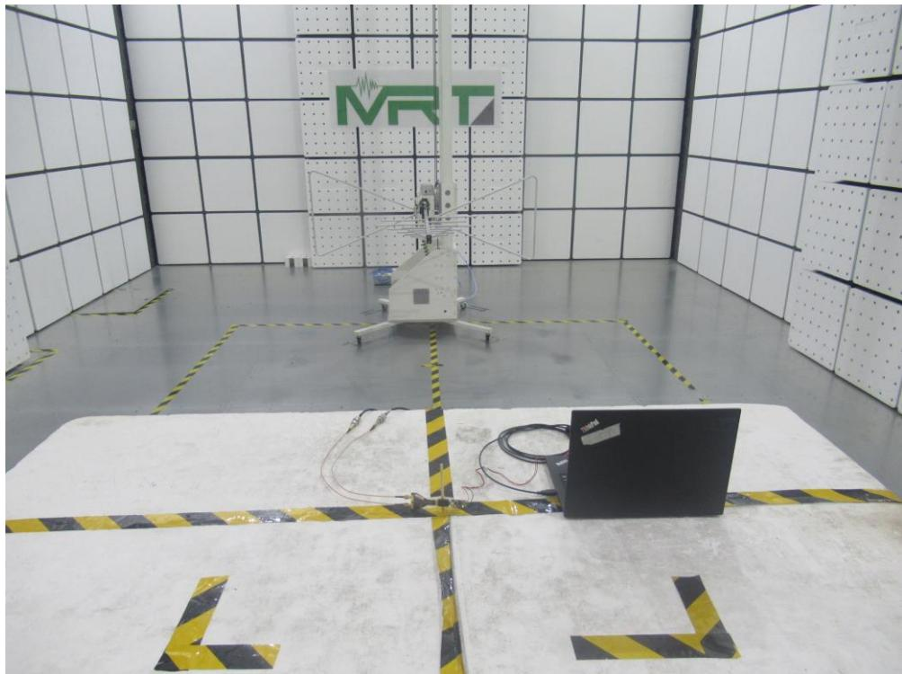
Description: Radiated Spurious Emission Test Setup for Below 1GHz(Low Rate)
