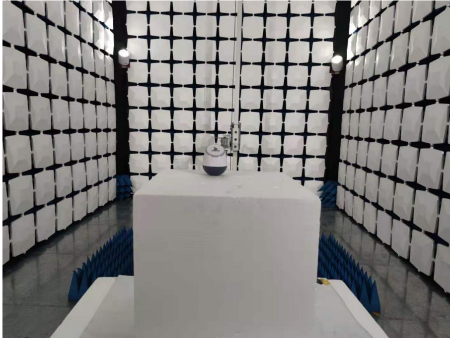
Above 1GHz for radiated emission test setup
