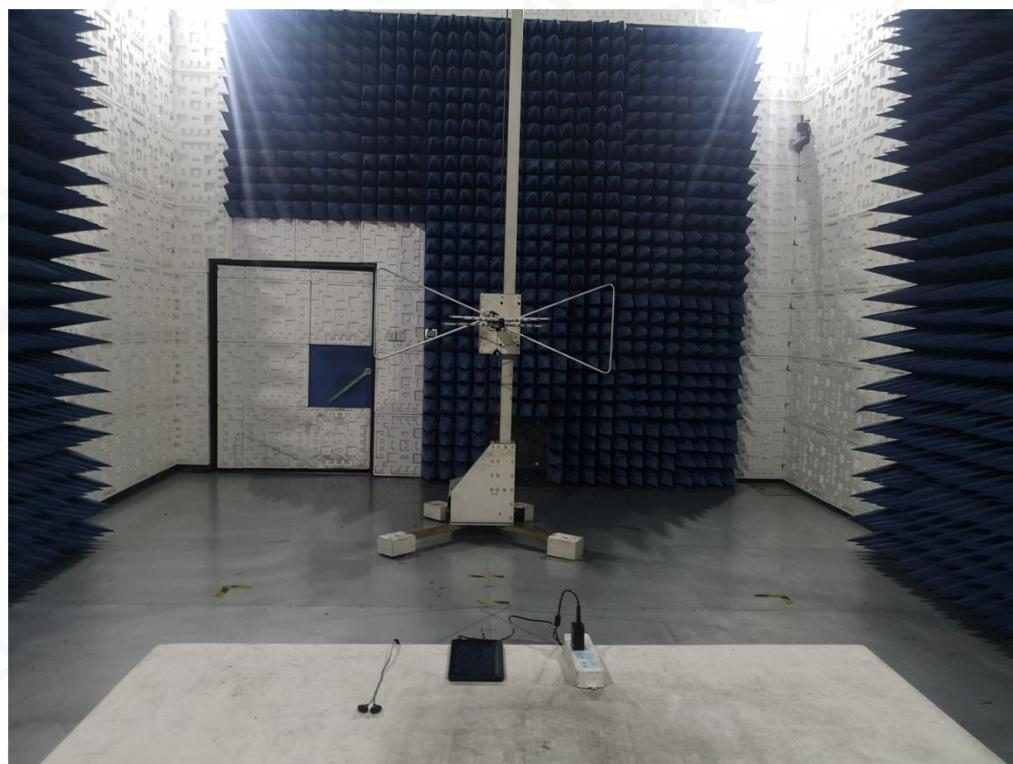
**FCC RADIATED EMISSION TEST SETUP ABOVE 1GHZ**
