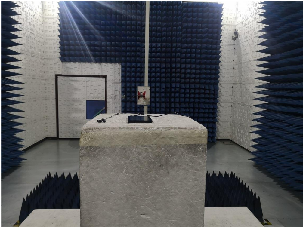
RADIATED EMISSION TEST SETUP ABOVE 1GHz
