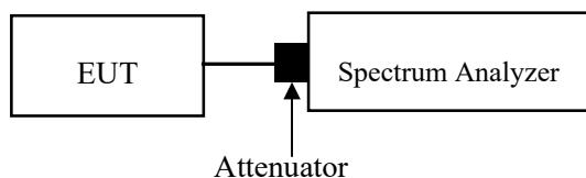
Note: A short RF cable with low cable loss connected to the EUT antenna port, which was provided by client or lab, the cable loss was add with offset into test equipment, the total offset consists of attenuator and/or RF cable loss
