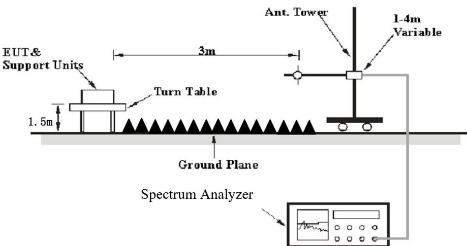
The radiated emission performed in the 3 meters, using the setup accordance with the ANSI C63.10-2020. The specification used was the FCC 15.209, FCC 15.247 limits.
