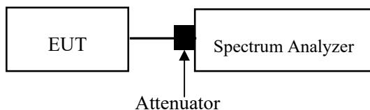
Note: A short RF cable with low cable loss connected to the EUT antenna port, which was provided by client or lab, the cable loss was add with offset into test equipment, the total offset consists of attenuator and/or RF cable and/or power splitter loss.
