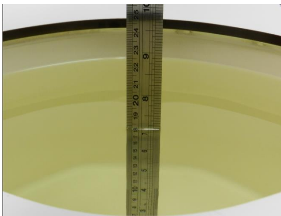
Fig 10.1 Photo of Liquid Height for Body SAR
