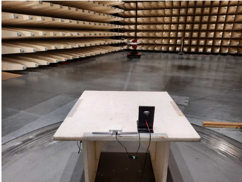
Photo 3: Chamber F below 1 GHz - without RFID TAG
