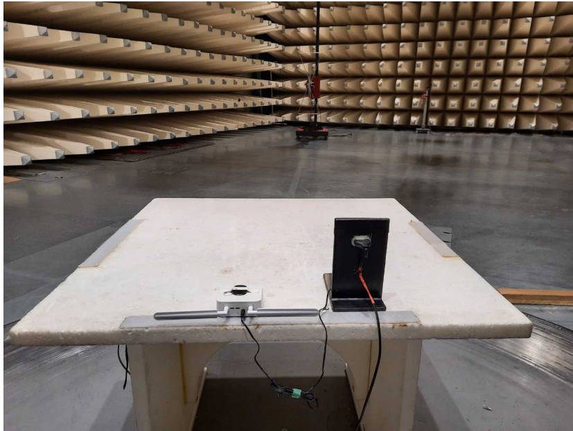
Photo 1: Chamber F below 1 GHz - with RFID TAG
