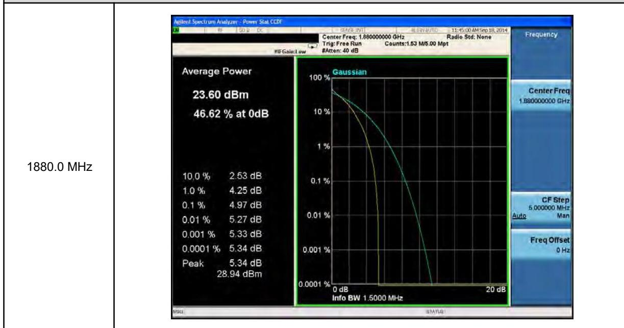
LTE Band 2 (Channel Bandwidth: 3 MHz) \_ QPSK
