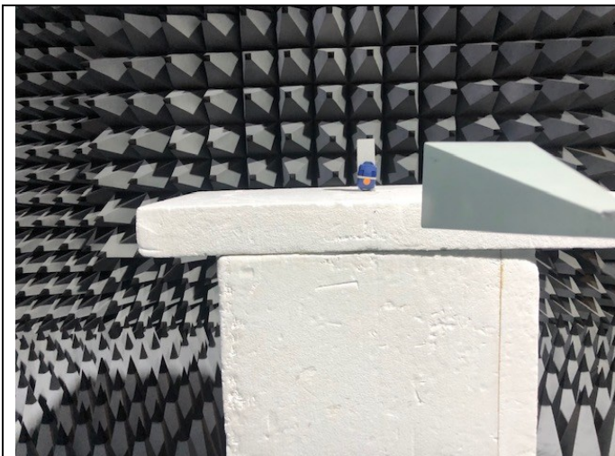
Fig 4 Test setup 18GHz 26GHz Rad Emissions
