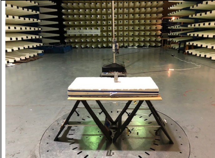
Fig 2a Test setup 300MHz -1GHz Rad Emissions
