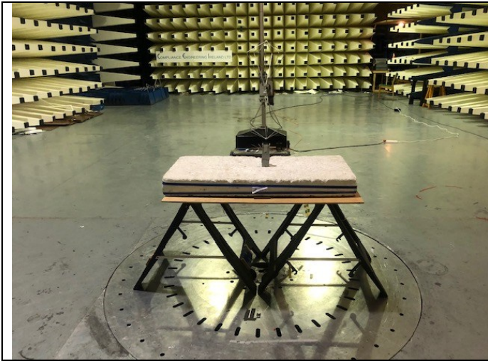
Fig 1a Test setup 30MHz -300MHz Rad Emissions
