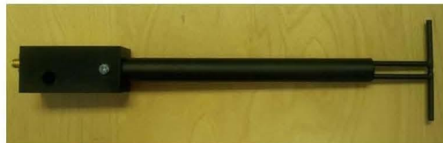
Figure 1 – MVG COMOSAR Validation Dipole
