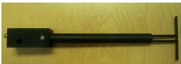
Figure 1 – MVG COMOSAR Validation Dipole
