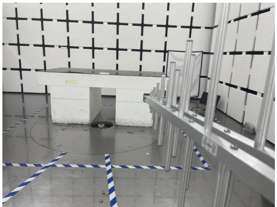
Radiation Emission Test Setup (30MHz to 1GHz)
