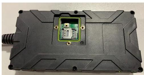
**Statements and Warnings:** The device card cover is locked with special screws, and can only be opened by professional installation tools and installation personnel.
