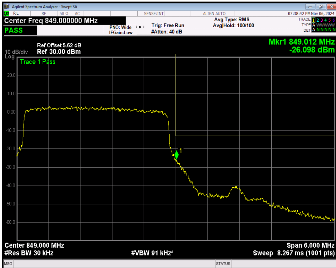
Band26(824-849) QPSK BW=5MHz Channel=26815 RB Size=25 Position=#0
