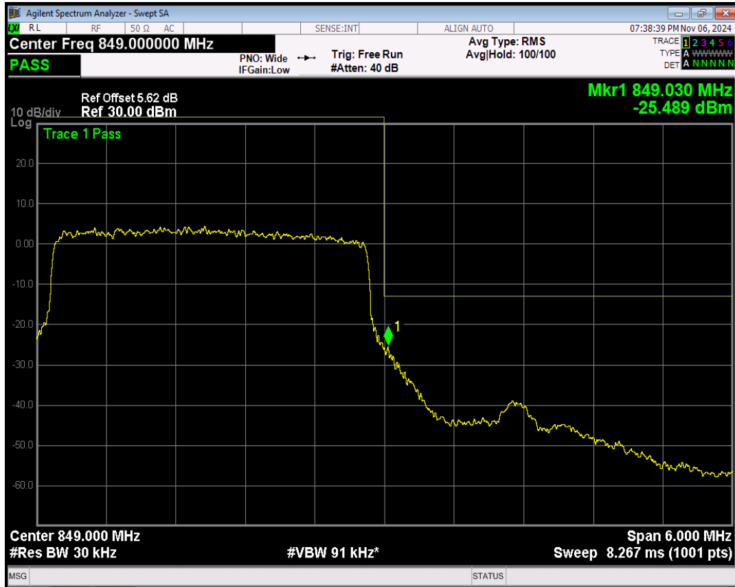
Band26(824-849) 16QAM BW=3MHz Channel=27025 RB Size=15 Position=#0
