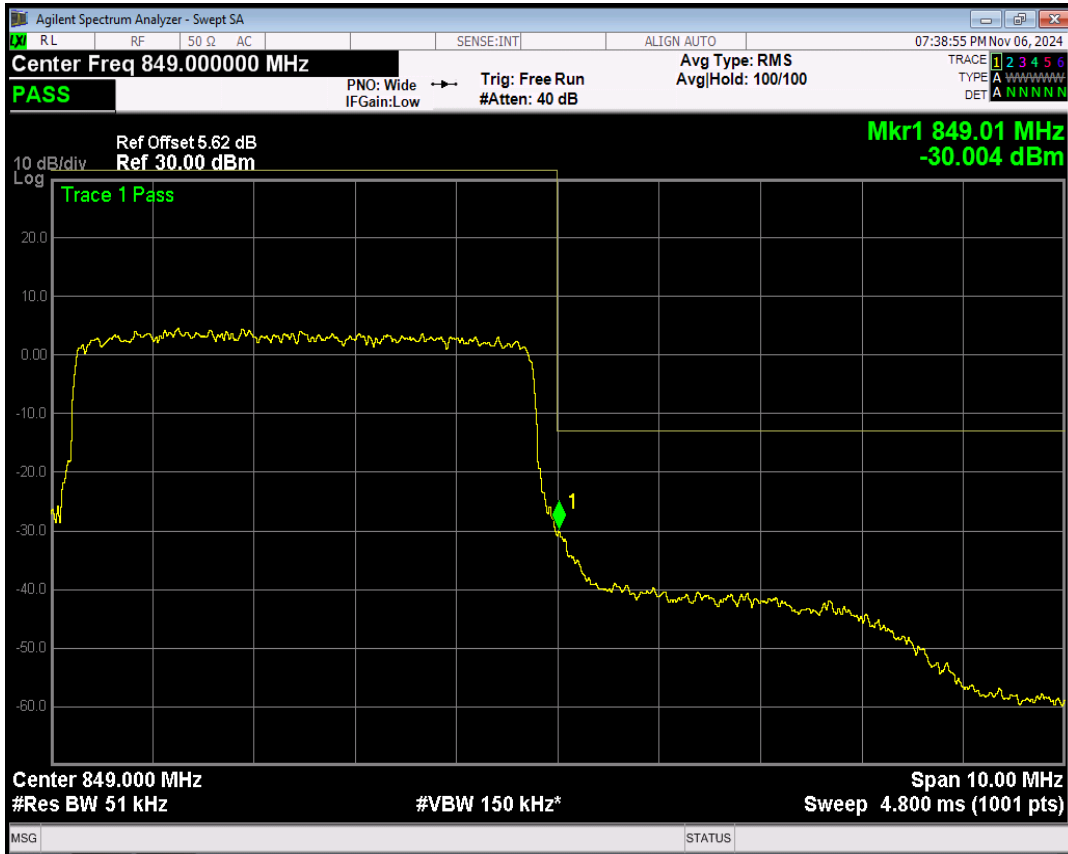
Band26(824-849) 16QAM BW=5MHz Channel=27015 RB Size=25 Position=#0
