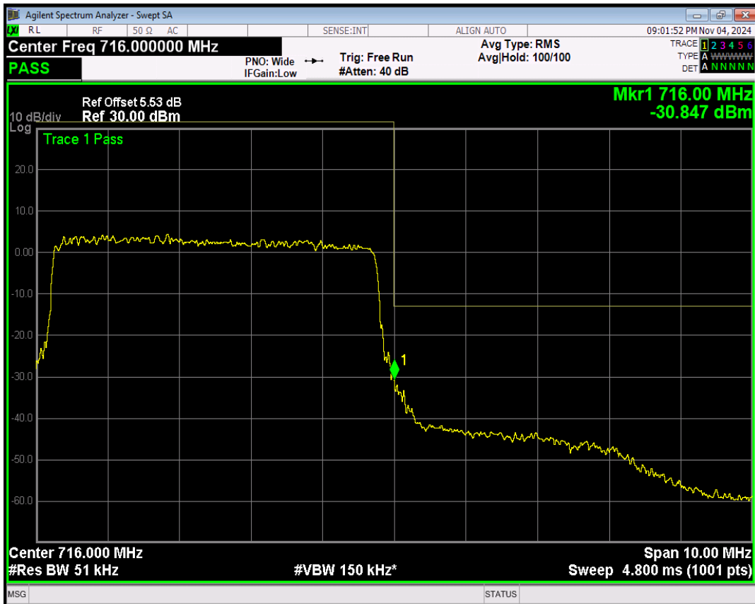
Band17 16QAM BW=5MHz Channel=23825 RB Size=25 Position=#0
