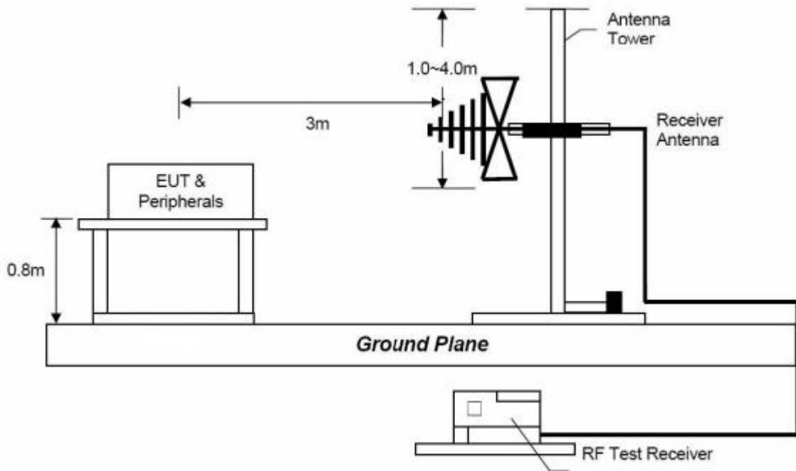
**Radiated Emission Test Set-Up, Frequency above 1GHz**
