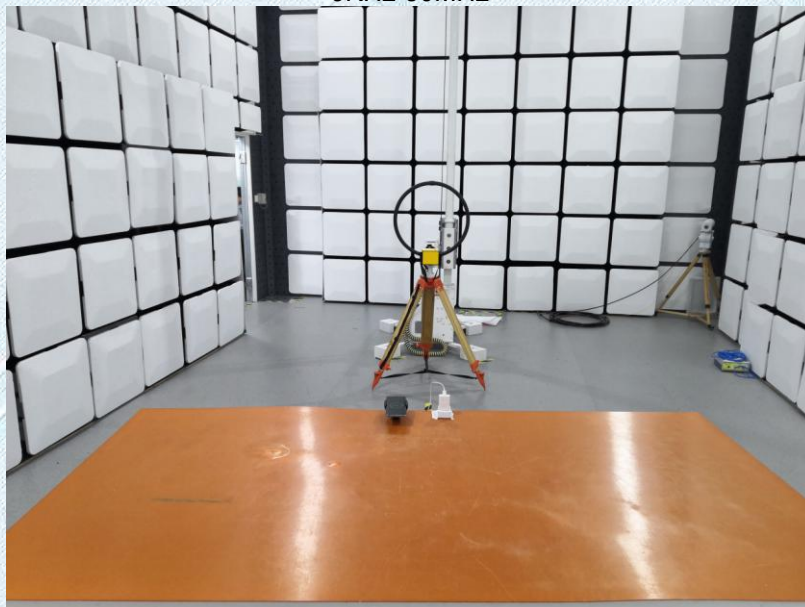
RADIATED EMISSION TEST SETUP 9KHz-30MHz
