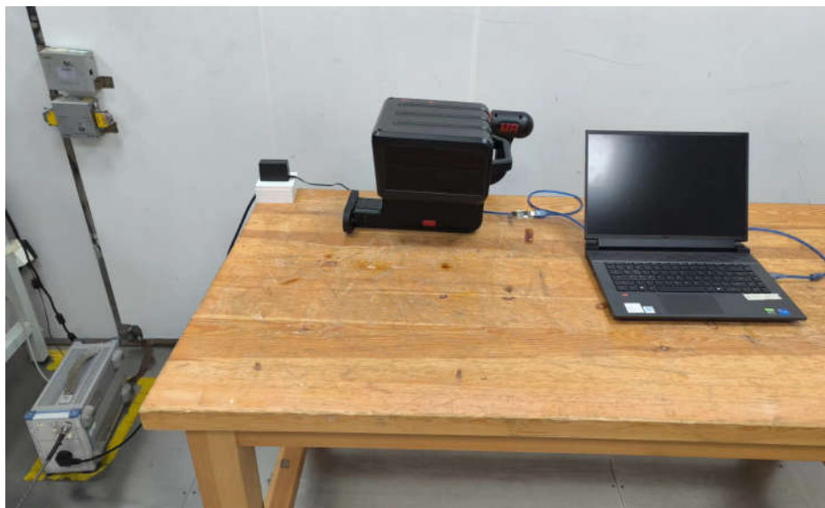
Conducted Emissions Test Setup-2
