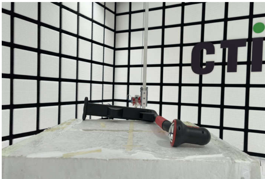
Radiated spurious emission Test Setup-3(Above 1GHz)
