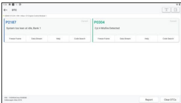
**⚠ Warning:** Reading fault codes when troubleshooting a vehicle is only a small step in the overall diagnostic process. Vehicle fault codes are provided as a reference only and parts cannot be replaced directly based on the fault code definitions given. Each fault code has a test procedure, and the service technician must strictly follow the operating instructions and procedures described in the vehicle service manual to identify the root of the malfunction.
