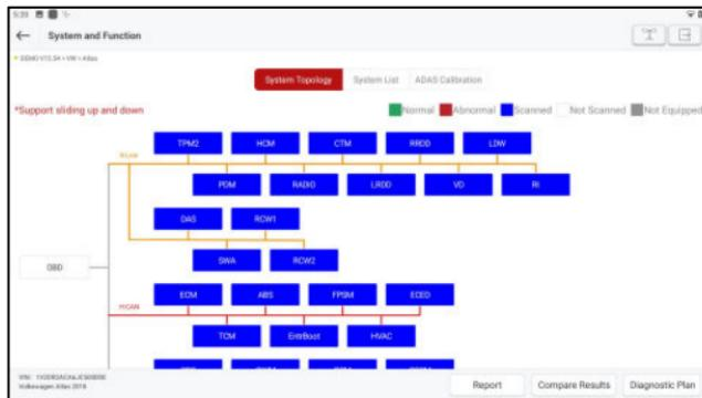
Users can manually select the vehicle electronic control system for test function operation. Click a single electronic control system (e.g. "ECM") in the test item selection interface, and then click "ENTER" to go to the test function selection page.
