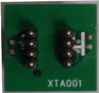
XTA001 | EEPROM chip adaptor                  | To place the EEPROM chip onto the adaptor, and then plug it into the programmer socket.                                     |
