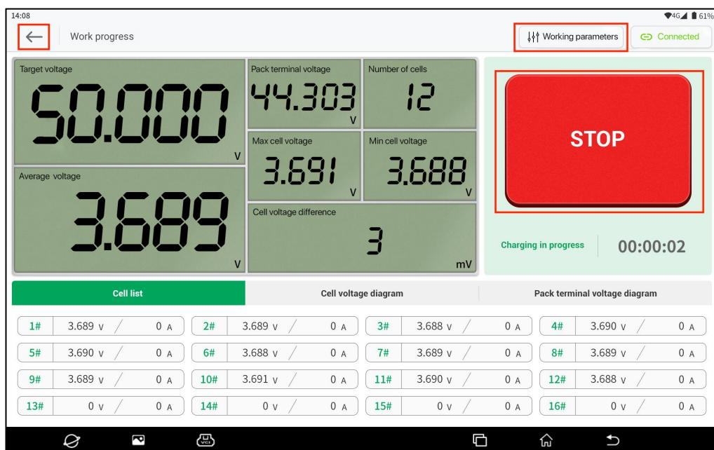
(7) Click the "View progress" button on the home page to switch to the operating progress screen, and click the "Stop" button to terminate the current charging/discharging process.
