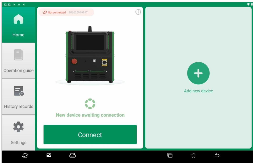
(6) When the buzzing sound indicates a successful connection, the device connection status shown before the serial number on the screen changes to "Connected." Click the "**Add new device**" button to add a new device in the same manner.
