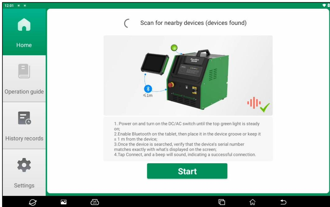
(5) Once the CE39 serial number is verified to exactly matches the serial number shown on the screen, click the "**Connect**" button.
