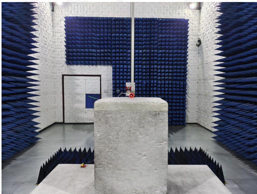
RADIATED EMISSION TEST SETUP ABOVE 1G
